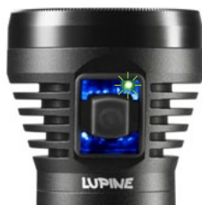
Battery voltage (once per 1/10 Volt)
